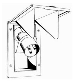
The external socket 220v - 16 Amps to CEE 17 (European Standards) is located on the external left hand side of the vehicle.
